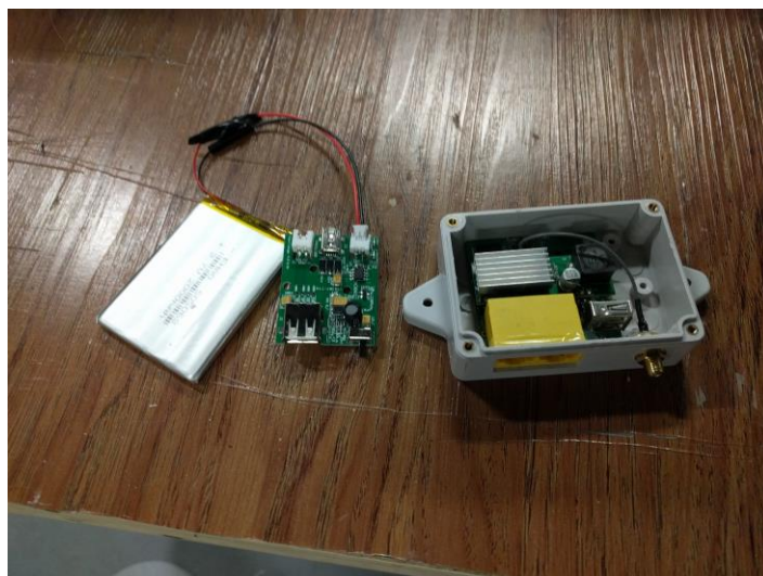
7: A 2,000mah Li-Po battery, charge controller, and AP150
